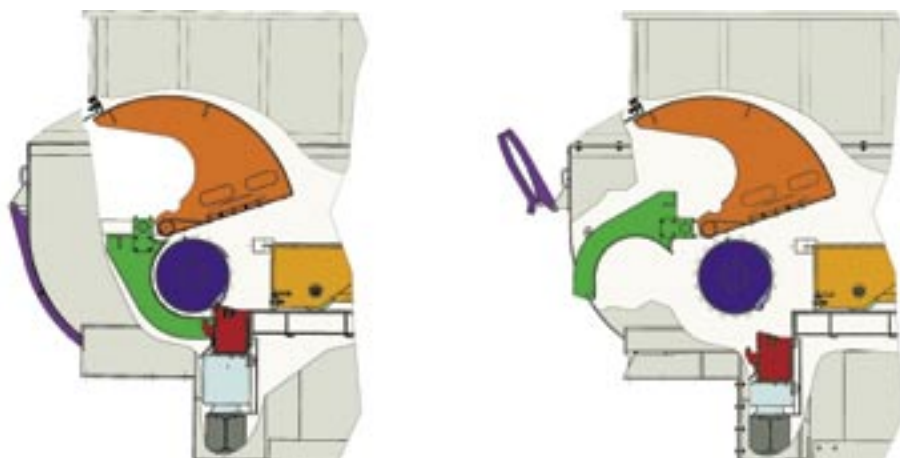
Fig 4—Optional movable screen unit is shown at left in the operating position, and in the open position at right, in order to clean between the shaft and the screen, or to replace the screen with one with different sized apertures.
